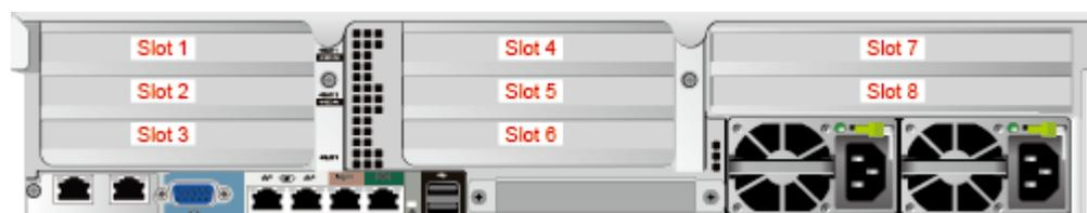
I/O module 1 provides slots 1 to 3, I/O module 2 provides slots 4 to 6, and I/O module 3 provides slots 7 and 8.
